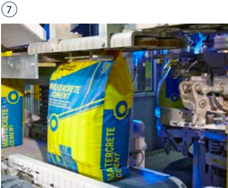
The full-bag transport The filled bags are forwarded in an upright position, closed and placed on the conveyor belt.
