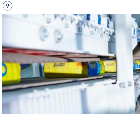
The bag forming section The belt conveyor consists of various adjustable elements, that ensure proper filling and increase process reliability. By using a pressing belt, the filled and sealed bags are formed precisely and can thus be palletized perfectly.
