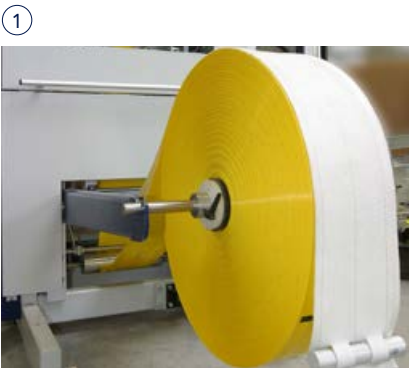
The tubular film The polyethylene bags are delivered as film (PE side gusseted tubular film) on rolls, picked up on a carrier and fed manually into the machine.
