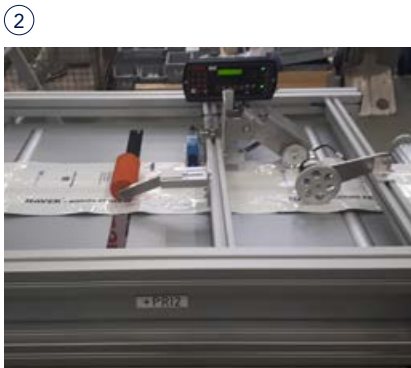
The printing The versatile marking systems ensure reliable and positionally accurate printing with your individual marking. We adapt this process step exactly to the speed requirements of the machine. Empty bag printing with laser (CO 2 + fiber laser), thermal transfer or labeler and full bag printing with inkjet are optionally available.
