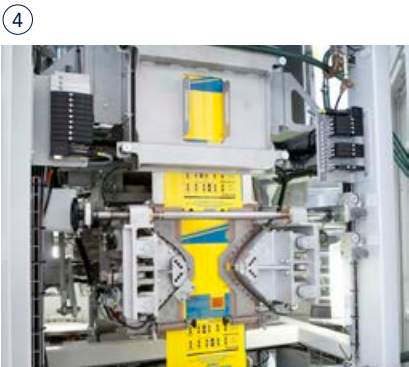
The bag manufacturing: corner welding and bottom seam welding Due to the diagonal welding of the side gussets, the bag bottoms are optimally formed. Among the advantages of corner welding are improved bag geometry, higher bag strength and very good stackability. This attractive positioning options on pallets, both in terms of storage positioning options on pallets. The machine automatically adjusts to different bag lengths as soon as the corresponding data have been entered. The system variably compensates for the bag lengths. Separated by a knife the bag is open at the top.
