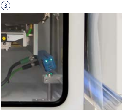
The bag scanner The optional bag scanner scans the QR code printed on the film to ensure that the machine operator is using the correct bag roll selected for the product to be filled. QR codes can additionally be used for product and bag tracing.
