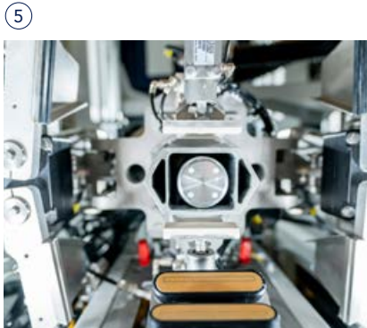
The hexagon filling spout The bag gripper clamps the bag chest tight to the hexagonal filling spout, reresulting in a clean filling process.
