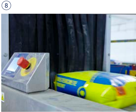
The quality control The check-weigher for the „bag-check“ with weight and closure control.
