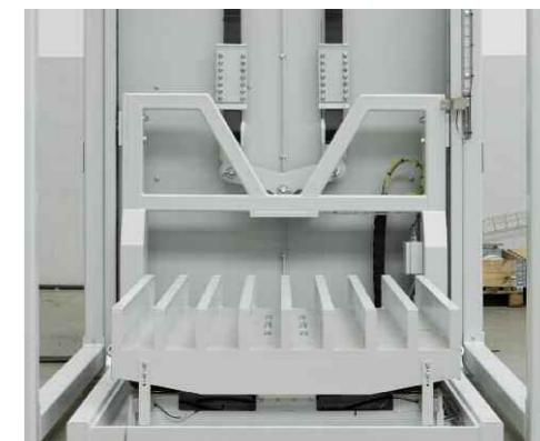
Movable compaction station with belt drive
