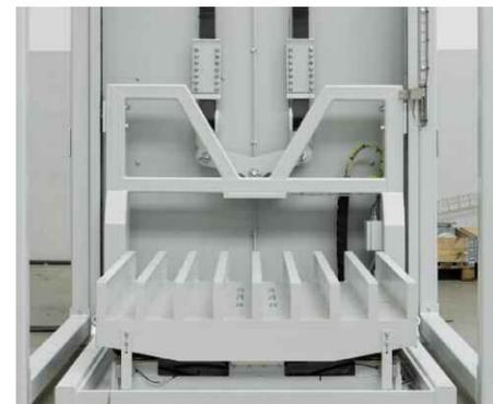
Movable compaction station with belt drive
