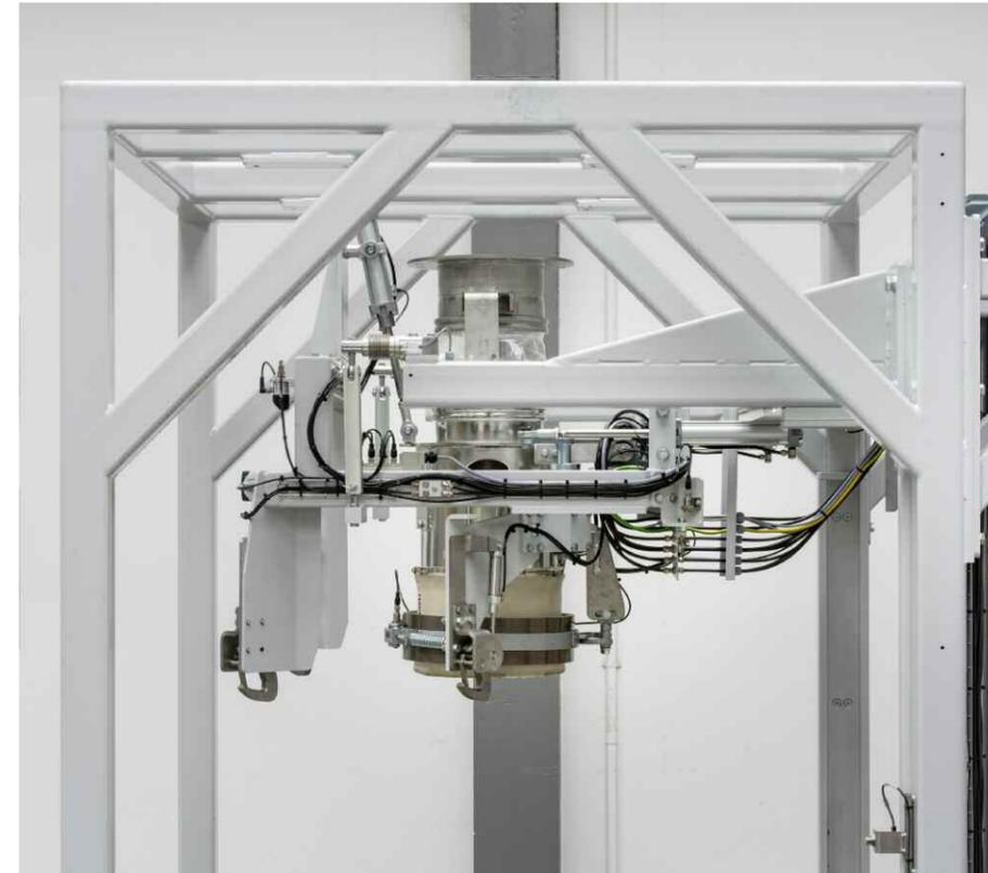
Side view of filling head and weigher cells
