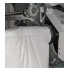
Spillage rejecting flap during filling process
