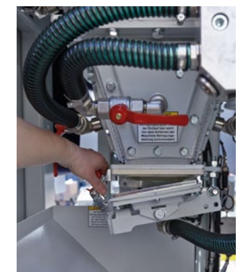
Maintenance flap at the filling box chamber
