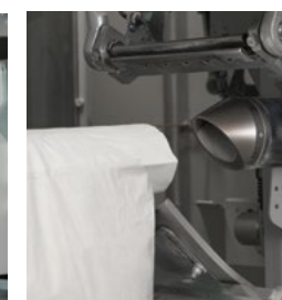
Spillage rejecting flap during bag discharge
