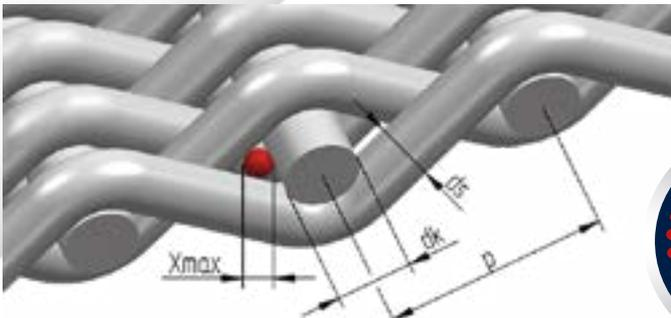
In the case of a twilled weave, the particle must pass through a pore channel. The decisive factor is the geometrical pore size ( $X_{\max}$ ).
