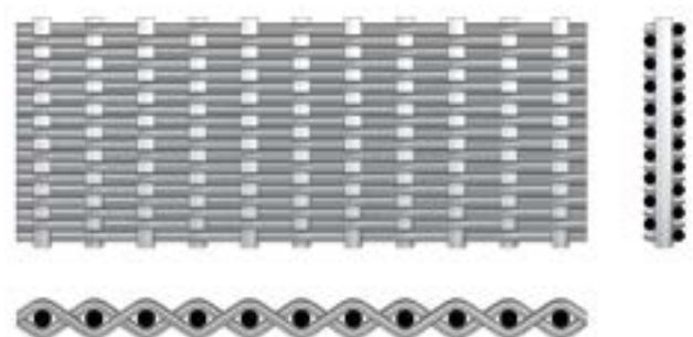
In the case of twilled weaves, the warp and weft wires are situated as tightly next to each other as possible.
