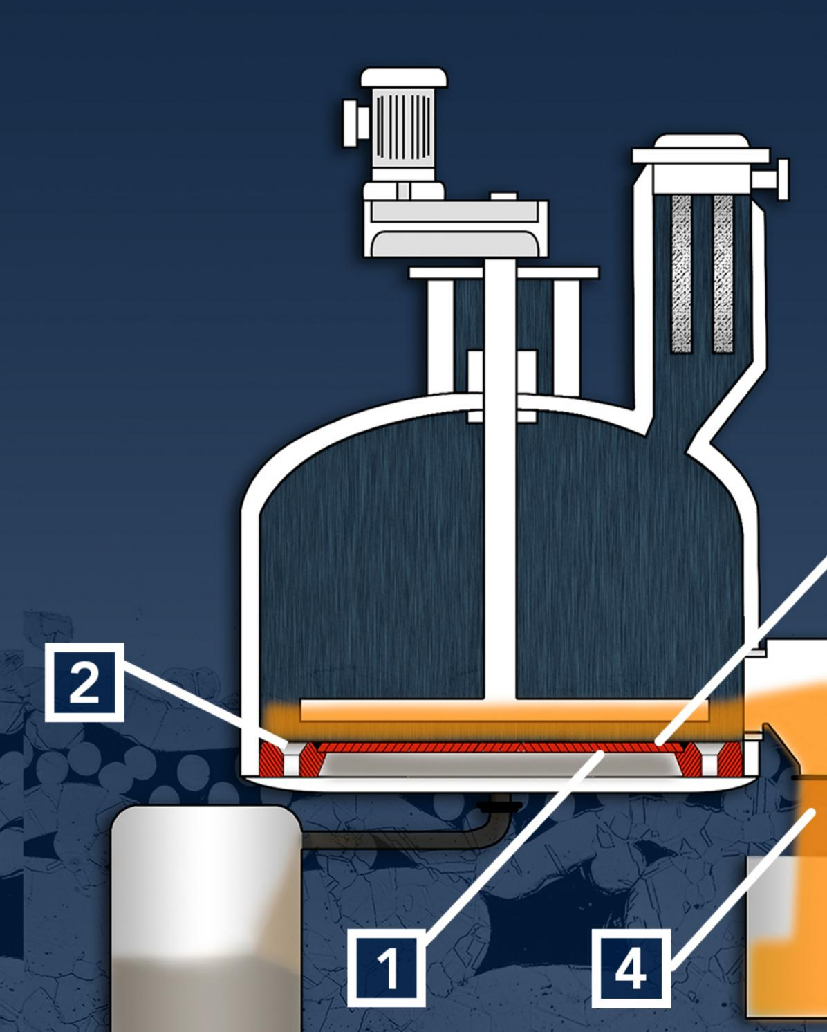
Avoid pressure to the bottom of the nutsche from the underside if the nutsche is not designed for a backwashing process:
