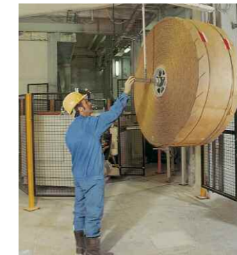
RADIMAT® system design with reel magazine and empty bag handling with reel system
