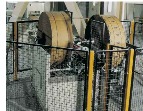
RADIMAT® system design with reel magazine and empty bag handling with reel system
