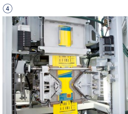
The bag manufacturing: corner welding and bottom seam welding
