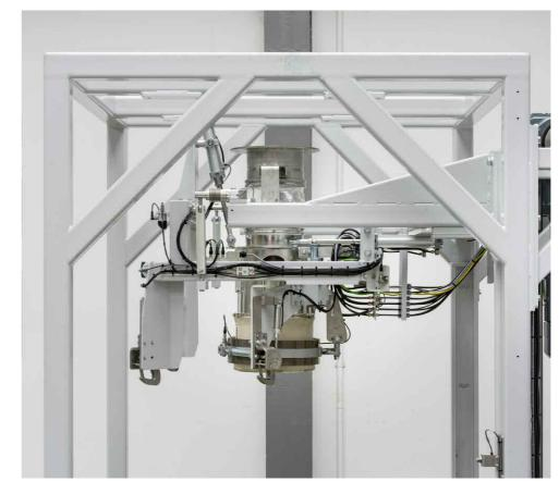
Side view of filling head and weigher cells
